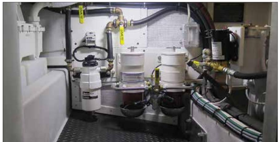
Generous utility space around the main engine installation provides easy access and encourages frequent maintenance of onboard systems like the fuel filters seen here. Much of that elbowroom was secured by forgoing an onboard generator in favor of solar panels.
