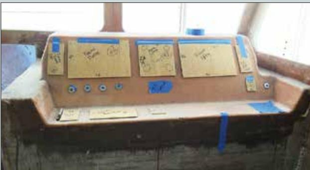
Workman advocates for having the customer on board to see and touch actual mock-ups in plywood and blue tape before making final installations.
