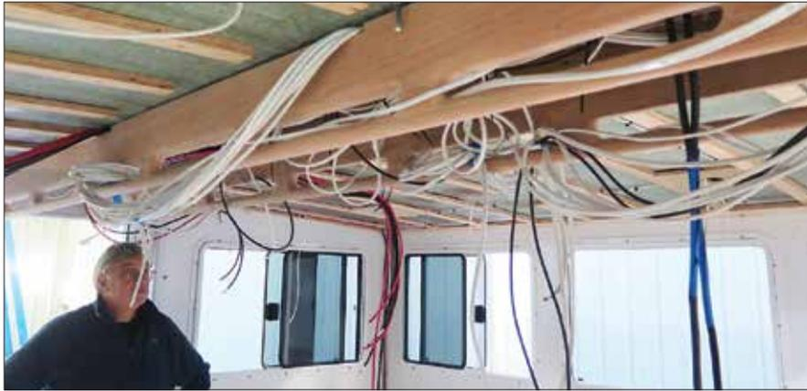
*As master electrician, Sigel oversaw installation of the complex wire runs in the pilothouse. After the overhead is finished, only the full-length longitudinal grabrails will be left exposed.*
