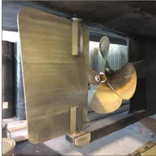
**Above**—A single prop and a skeg-hung rudder are in *Star*’s workboat DNA and on Sigel’s priorities list. **Right**—Workman suggested the QSC 8.3 diesel based on Sigel’s speed and sound requirements, and the fact that in any single-engine installation, reliability and simplicity are essential.
